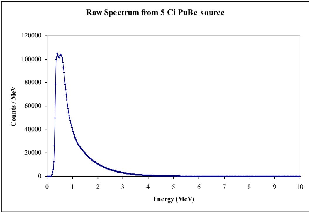
FIGURE 2: The raw neutron spectrum collected from a 5 Ci plutonium-beryllium source
