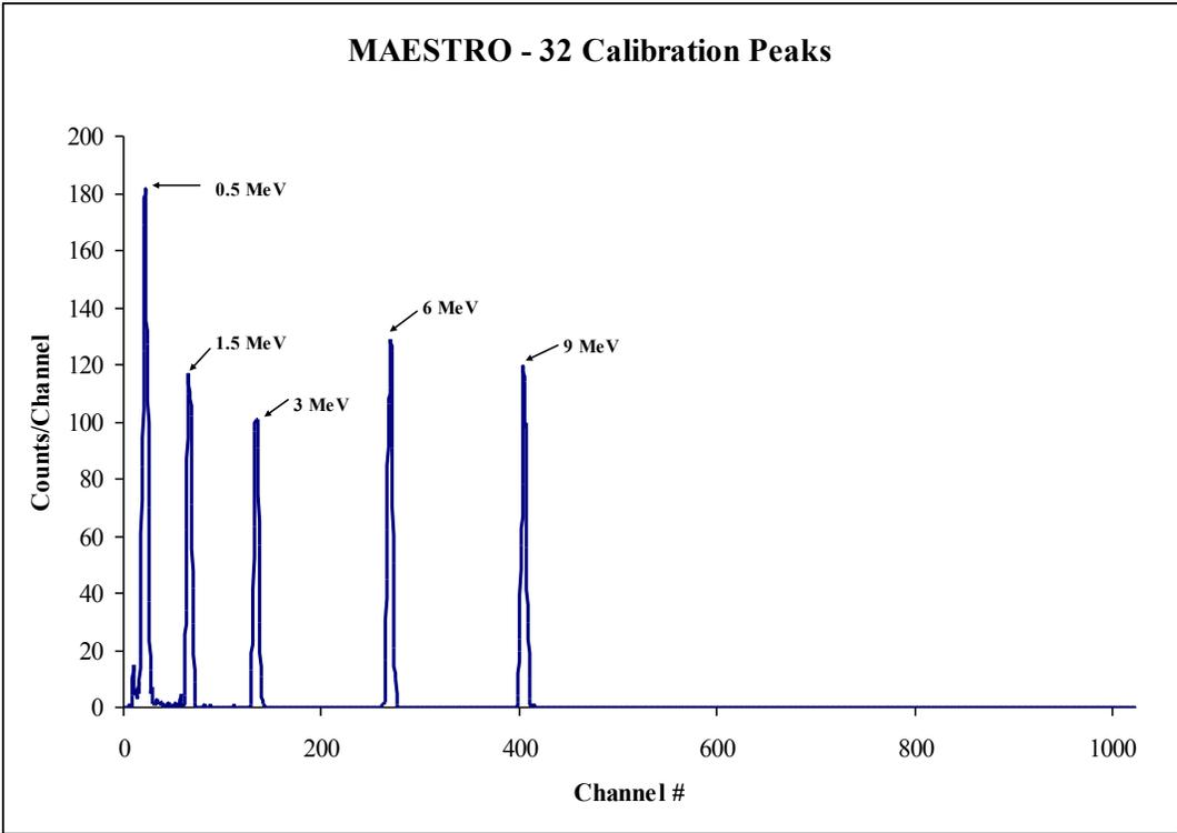
FIGURE 3: Peaks produced in the pulser for use in the energy calibration procedure
