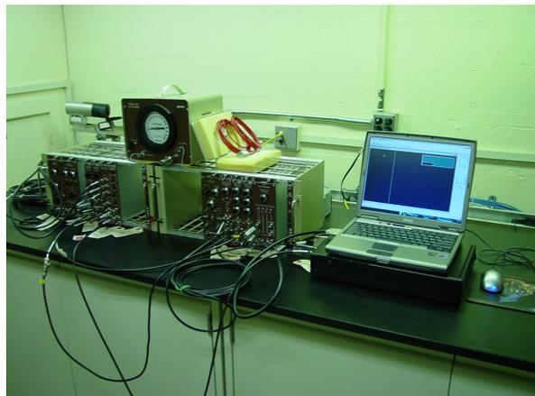
**FIGURE 1:**  $^3\text{He}$  spectrometer with PCI expansion box and Dell Laptop used for data collection
